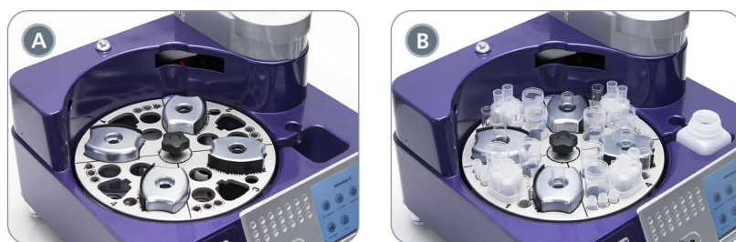
Figure 5. Carousel Quadrants. All four quadrants (A) empty and (B) loaded.
