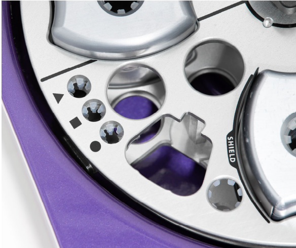
Figure 6. Carousel Gaskets. Gaskets at reagent vial and sample tube locations.
