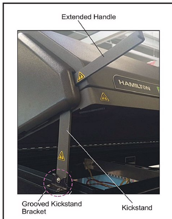
Figure 27. Secured Kickstand in Bracket with Handle Extended
