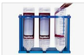
Add density gradient medium to SepMate™ tube, then rapidly pipette or pour the blood sample directly over the insert.
