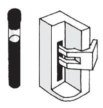
2. For magnetic separation, place the test tube in the Dynal MPC-1 and ensure that the clamp holds the tube in place.
