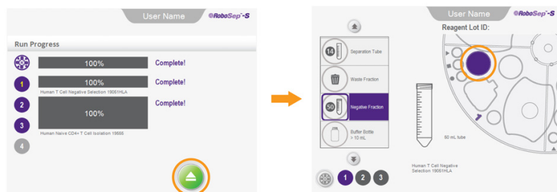
Figure 22. Collecting Isolated Cells at the End of a Protocol Run. The desired isolated cells are located in the tube highlighted in color in quadrant #1 of the Unloading screen.
