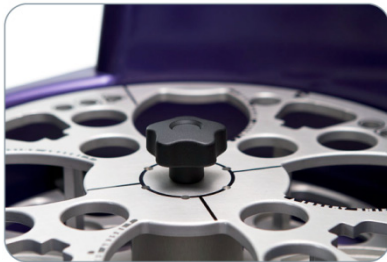
Figure 23. Black Central Knob Used to Remove the Carousel.
