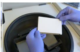
Align the absorbent paper with the edges of the BaseFrame.
