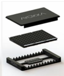
The system consists of three components (from bottom to top): the LUNARIS™ BaseFrame, 1–4 BioChips and a lid. The BaseFrame enables assays in 96 or 384 MTP-formats by rotating the frame 180 degrees.
