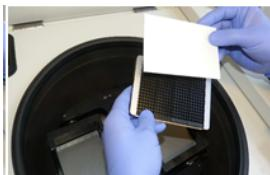
Place a sheet of absorbent paper (provided with the kit) on top of the assembled LUNARIS™ BioChip.
