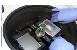
Position the assembled unit in a plate centrifuge.
